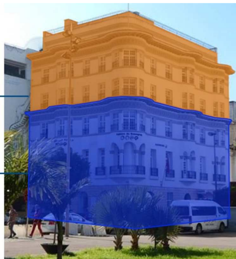
Figure 5: Schematic Illustrating the Intervention of Façadism on the Building «Le Gourmet», Rabat. Karima BERDOUZ, 2018.
